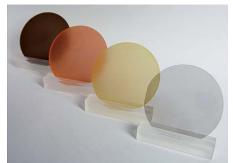
The different colour nuances of the AlYN/GaN wafers visible here result from different yttrium concentrations and growth conditions.
