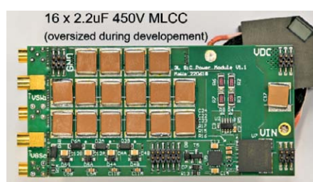
Figure 3: Technology demonstrator platform: Physical PSU mainboard (270 x 83 mm², 22 mm height) with 2x interleaved 3-level flying capacitor HF legs for PFC, which are 32 x 60 mm² in size.
