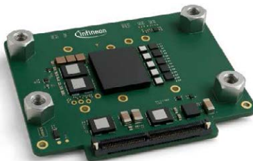
Figure 5: Example circuit of a HV IBC from 800 V to 50 V with 6kW (Image: Infineon Technologies)
